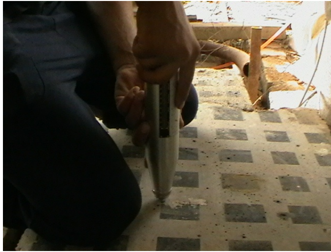
Plate.2 Rebound Hammer testers
