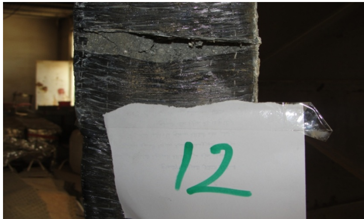
B- Failure mode for specimen NF-10H100
