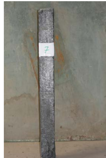
B- Column (0.75SF100-12H100) after rehabilitation
