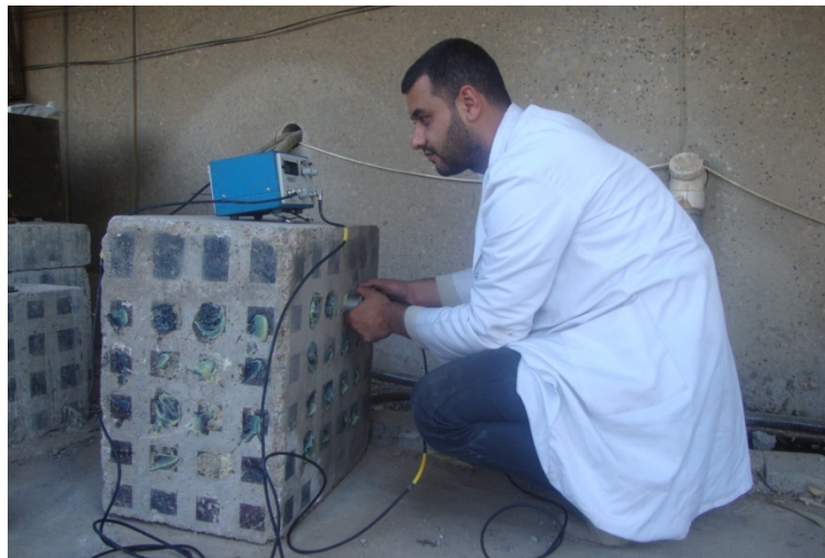
Plate.1 Direct and Indirect Reading of Ultrasonic Pulse Velocity
