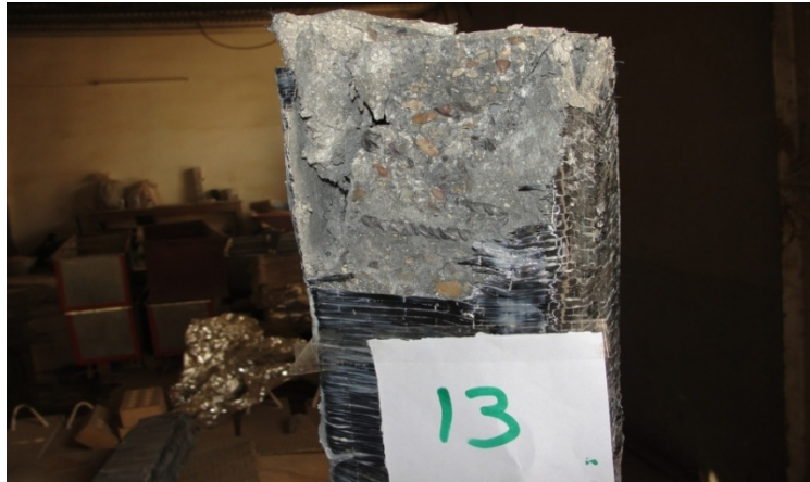
A- Failure mode for specimen NF-8H100
