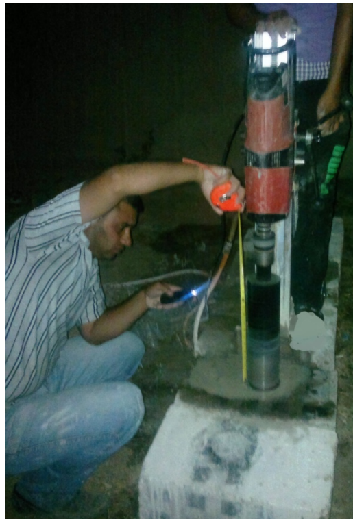
Plate.3 Cutting core specimens from Beam sample
