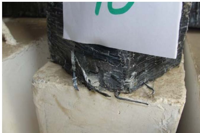
C- Failure mode for specimen 0.75 SF100-10H100
